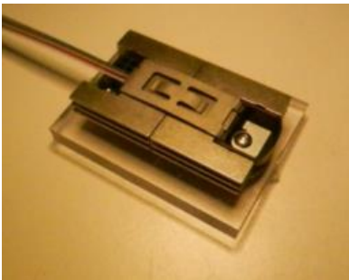
2way optical engine assembly with heat sink and optical cable
